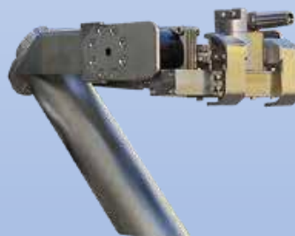
HYDRANT TOOL FOR HIGH FLOW OR HIGH PRESSURE DIRECTIONAL WATER JETTING
